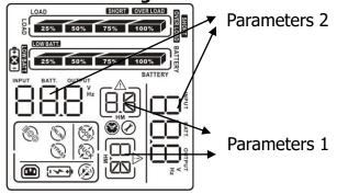
There are two parameters to set up the UPS.
