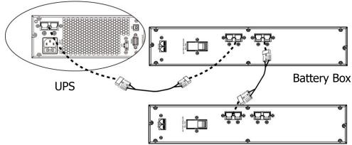
**NOTE:** Maximum connected external battery boxes up to 4 units.
